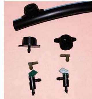
Individual drip emitters apply water at a given rate to a specific location. Emitters are typically rated at 1 – 4 gallons per hour. Emitters are usually attached at the end of a 1/4" tube that is connected to the main supply line. Some emitters are pressure compensating and can be connected to higher-pressure lines or to lines that have variable pressure due to changes in elevation. Other emitters must have the supply pressure reduced in order to function properly.
